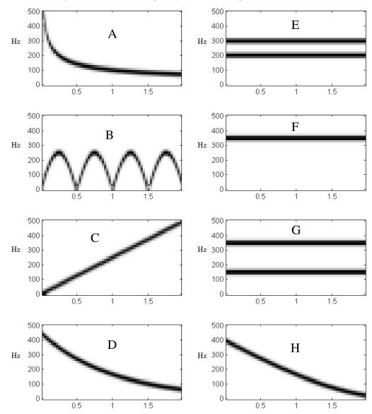
**PROB. Fall-12-Q2.2.** Shown below are the spectrograms (labeled A through H) for eight signals over the time range  $0 \le t \le 2$ . The frequency axis for each plot has units of Hz.
