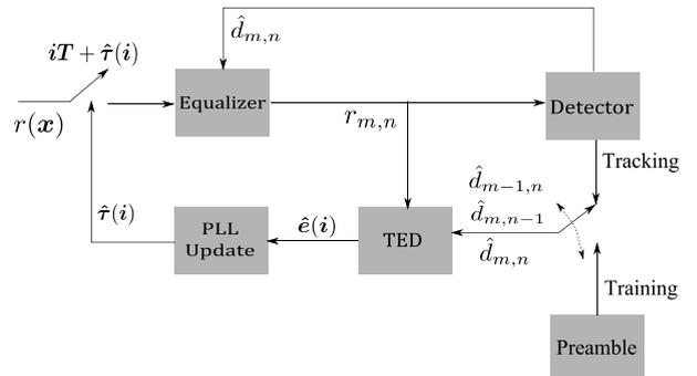
**Fig. 19. Architecture of the 2-D PLL. The timing estimates  $\hat{\boldsymbol{\tau}}(\mathbf{i})$  are used to correct the sampling instants at  $\mathbf{i}^T \mathbf{T}$  [92].**
