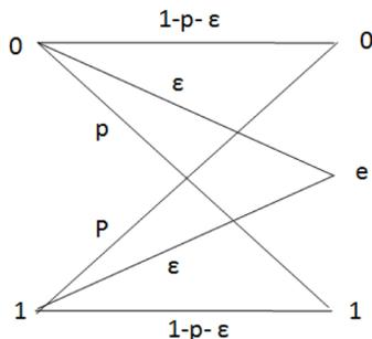
**Fig. 2.** The representation of binary error and erasure channel model.
