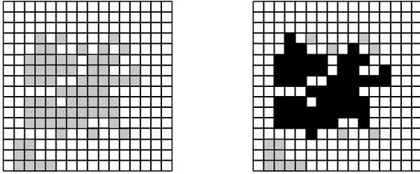
**Fig. 30.** Two-dimensional defective regions on a medium are identified within a largest edge connected region. These are later flagged as erasures and corrected using an LDPC code and a channel detector. (a) 2D defective regions. (b) Identified rectangular bursts.
