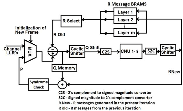
Fig. 32. Block diagram of the layered decoder.
