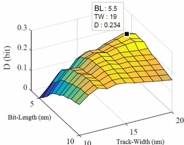
**Fig. 13.** Finding the optimal TW and BL by maximizing information rate per grain  $D$  for the TDMR<sub>2</sub> system with the parameters provided in Table 1. The MIR for maximum  $D$  is found to be empirically approximately 0.6 under these conditions.
