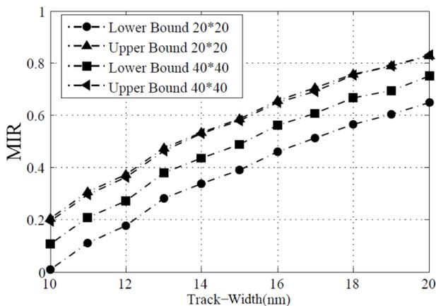
**Fig. 12.** Lower and upper bounds on the MIR of the TDMR<sub>1</sub> system with the Voronoi channel model. It is shown that increasing the track width decreases media noise leading to the MIR increment.
