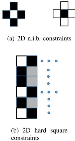
**Fig. 24.** Configurations of some 2-D modulation constraints. (a)  $3 \times 3$  n.i.b constraints juxtaposed side by side with a base pattern and its complement. (b) Two-dimensional  $(1, \infty)$  RLL constraint: The white and black squares indicate a “+1” and “-1,” while a gray square can be either “+1” or “-1.” The bits are populated within the array with the above constraints.
