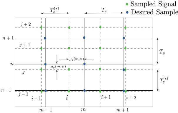
**Fig. 21.** The sampled points of the read-back signal  $j_T$  and the desired samples are at the intersections of the dotted and solid lines. The interpolation filter attempts to estimate the samples at the desired points from the sampled signal.
