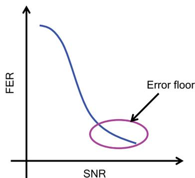
**Fig. 28. Illustration of the “error floor” behavior of LDPC codes. Initially, as the SNR increases, there is a sharp downward slope as the FER decreases. However, this slope eventually levels off, leading to much smaller improvement in FER for high SNRs.**
