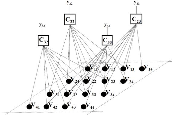
**Fig. 10. Factor graph of a  $4 \times 4$  lattice square of random variables  $\mathbf{V} = [V_{i,j}]_{i=1}^4, j=1}^4$  where every  $3 \times 3$  lattice square of variables is controlled by a local function  $C_{i,j}$ . The variable nodes  $V_{i,j}$  s are shown with circles and factor nodes  $C_{i,j}$  with squares where  $(i,j)$  and  $(i',j')$  specify the position of the node in the lattice square.**
