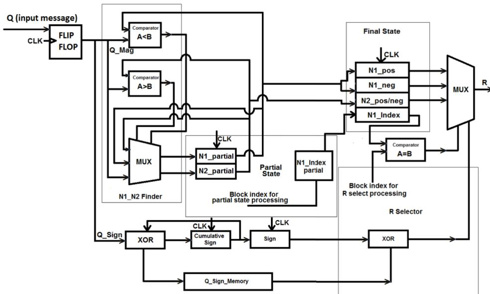
Fig. 33. Architecture of the CNU.  $Q$  and  $R$  represent the incoming and outgoing messages, respectively.
