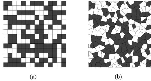
**Fig. 6.** Writing on the Voronoi-based media model (first method). (a) The resultant magnetization of an ideal medium. (b) The resultant magnetization of an actual medium. The grains with magnetization  $+1/-1$  are colored white and black, respectively.
