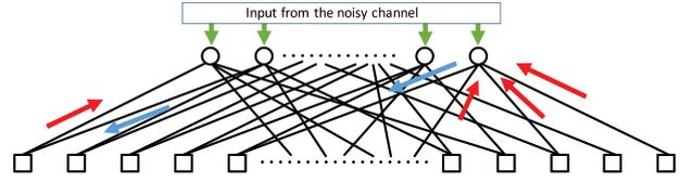
**Fig. 26.** A bipartite graph representation of an LDPC code. Variable nodes are marked in circles and check nodes are marked in squares. A check node is satisfied if the mod 2 sum of its neighboring variable nodes is 0.
