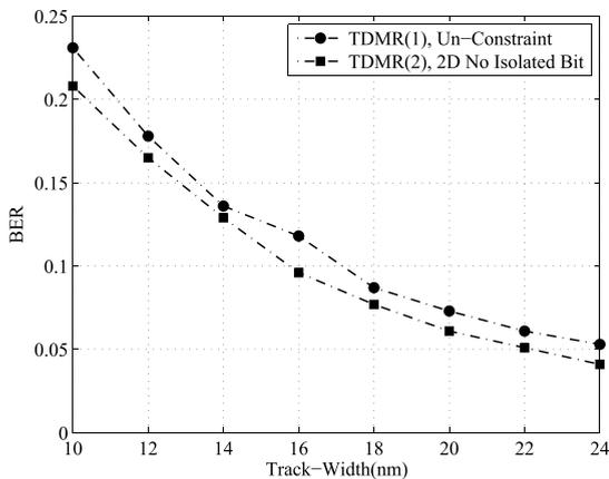
**Fig. 25.** BER comparison of uncoded [TDMR(1)] and coded [TDMR(2)] systems with different bit areas and the same storage density in absence of electronic noise. Constrained coding improves the performance by avoiding the data patterns that result in high media noise.
