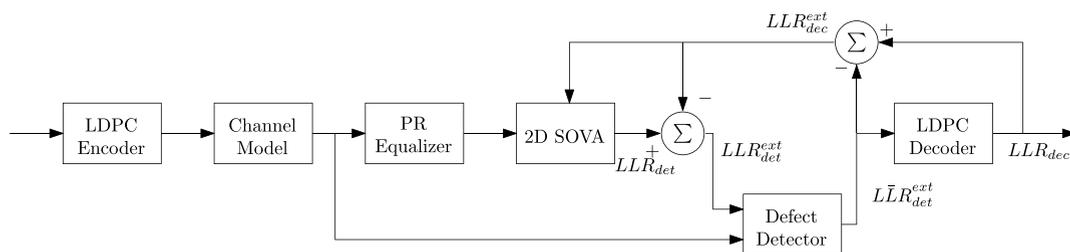
**Fig. 31.** Schematic of a defect detector and erasure decoder architecture for TDMR. The LLR values for bits identified as defects are set to zero in the channel detector. The LDPC decoder provides extrinsic information for these erasures. The detector and the decoder are iteratively configured to resolve the burst erasures.
