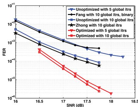
**Fig. 29. Performance advantage of using a code optimized for the PR setting (see [133]).**
