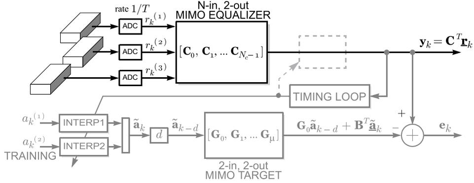
**Fig. 17. Signal processing architecture for multitrack detection with multiple readers.**
