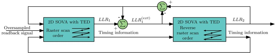
**Fig. 23. Turbo scheme for 2-D joint timing recovery and signal detection. The scheme uses two instances of the joint timing detection algorithm, where one instance operates in the raster scan order, and the other instance operates in the reverse raster scan order. The two instances exchange timing information, as well as extrinsic information to achieve overall improvements in bit error rate performance [97].**
