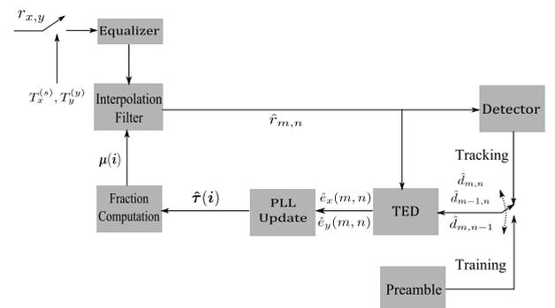
Fig. 20. Schematic architecture of the 2-D ITR scheme [96].
