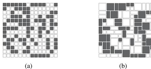
**Fig. 4.** (a) Ideal medium of size  $14 \times 14$ . (b) Example of a medium consisting of grains of sizes up to  $2 \times 2$  cells.
