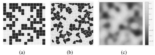
**Fig. 7.** Write/read model for the Voronoi medium. (a) Desired magnetization of an ideal medium. (b) Magnetization of a nonideal medium. (c) Read-back signal (before sampling). We assume the read-back impulse response to be a truncated 2-D Gaussian pulse of unit energy with half-maximum of 1 bit-period and a span of 3 bit-periods in both dimensions.
