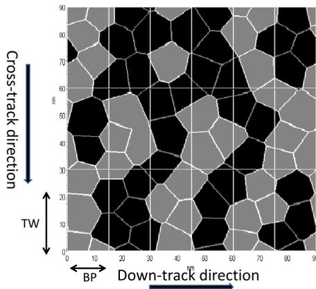
**Fig. 5.** An example of the Voronoi channel model for a TDMR system. We set the length of each bit cell in the horizontal (down-track) direction to be  $BP = 15$  nm and in the vertical (cross-track) direction to be  $TW = 30$  nm. The CTC parameter is considered to be 10 nm.
