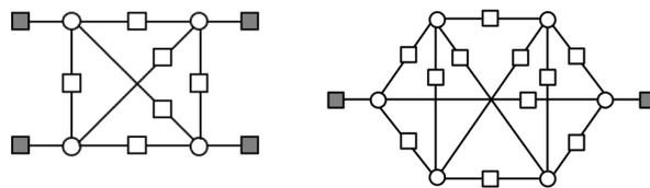
**Fig. 27. (Left) (4, 4) configuration. (Right) (6, 2) configuration. Circles denote variable nodes and squares denote check nodes. When the shown variable nodes are set to 1 (and all other variable nodes are set to 0), white checks are the satisfied checks, and black checks are the unsatisfied checks.**
