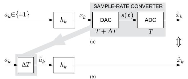
**Fig. 15.** Modeling frequency offset.
