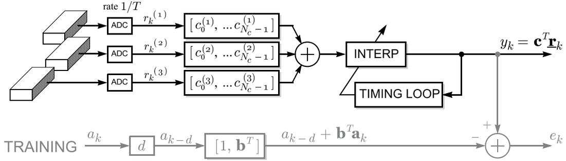
**Fig. 14.** Signal processing architecture for single-track detection with multiple readers.
