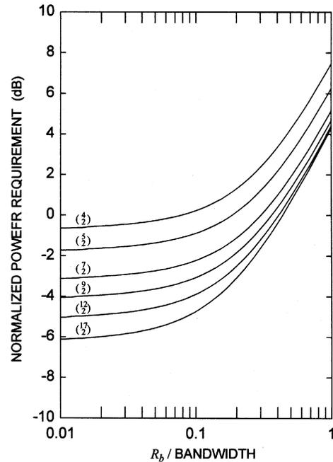
Fig. 2. Normalized power requirement versus normalized bit rate on an ISI channel with MLSD for MPPM.
