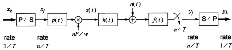
Fig. 1. Block diagram of MPPM system.
