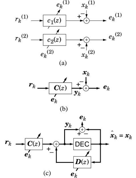
Fig. 2. Three adaptive receivers: (a) conventional receiver; (b) LE receiver; (c) DFE receiver.
