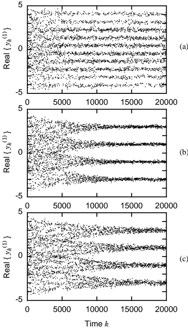
Fig. 4. Real part of first component of equalizer output for (a) vector CMA; (b) pointwise CMA; and (c) combination CMA.
