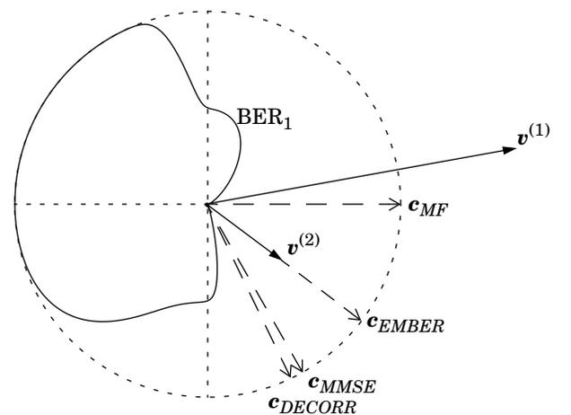
**Fig. 1.** A polar plot of  $\text{BER}_1$  versus  $\theta$  for a two-user system with correlation  $\rho = 0.9$ . Superimposed are the signal vectors (scaled by a factor of 0.5) and the MMSE, decorrelating, MF, and minimum-BER detectors.
