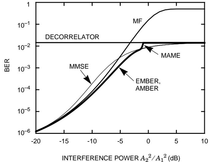
Fig. 4. BER versus normalized interference power.
