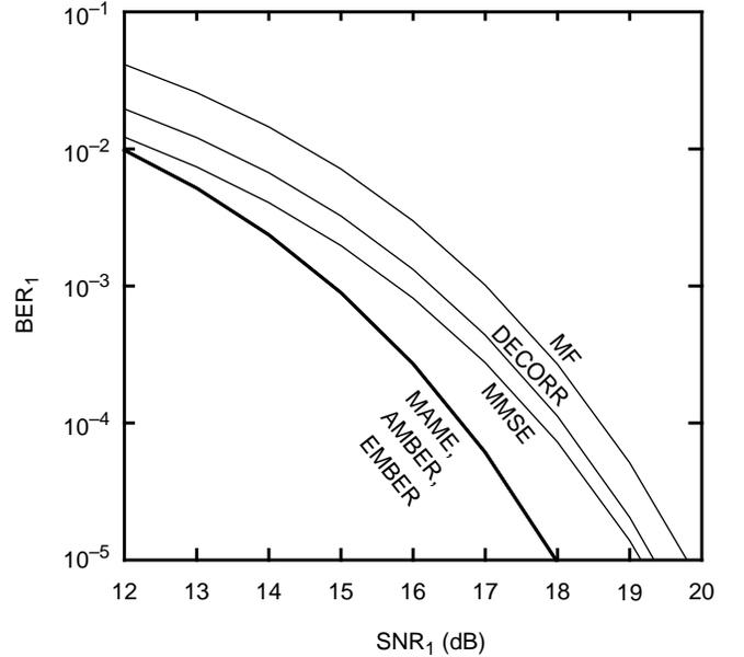
Fig. 3. Theoretical steady-state BER comparison.
