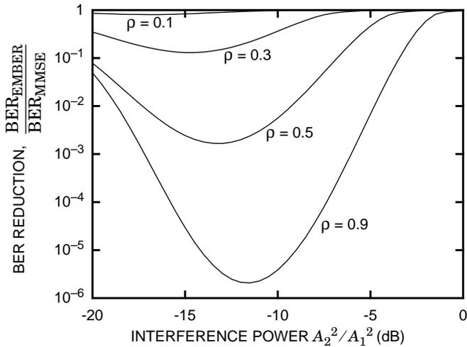
Fig. 2. A plot of  $\text{BER}_{\text{EMBER}}/\text{BER}_{\text{MMSE}}$  versus interference power for  $\text{SNR}_1 = 20$  dB.
