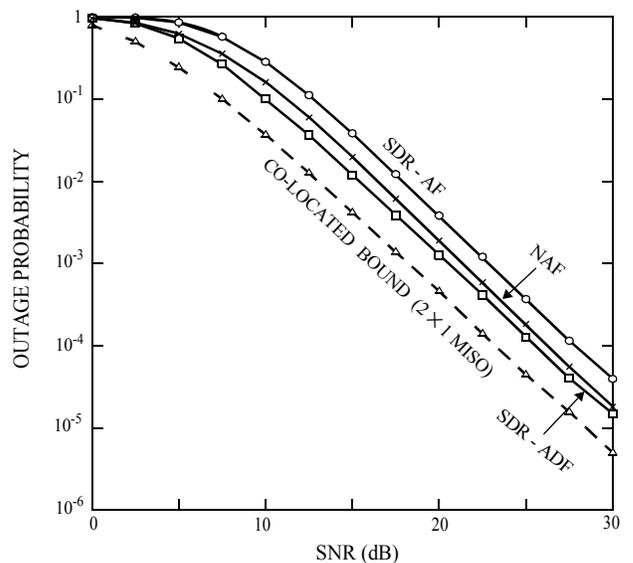
**Fig. 3.** Comparison of outage probabilities of non-orthogonal cooperation schemes for a 2-user system, with  $R = 1$  bps/Hz.
