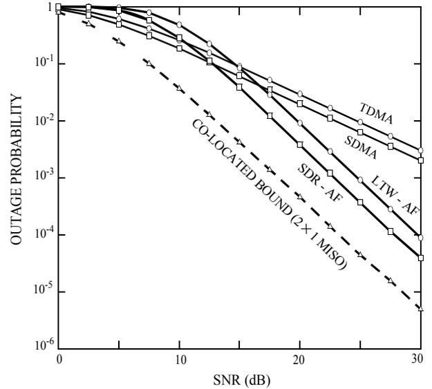
**Fig. 2.** Comparison of outage probabilities of various multiple access schemes for a 2-user system, with  $R = 1$  bps/Hz.
