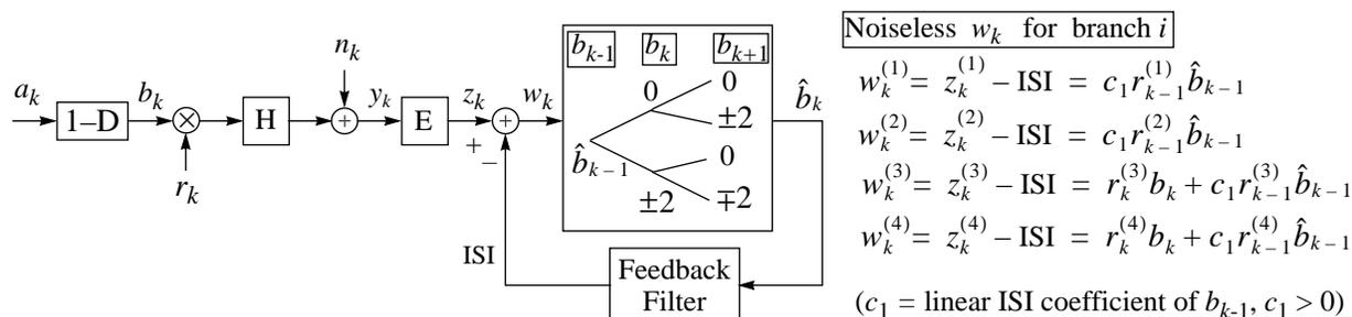
Figure 1: Partial erasure channel + FDTS/DF
