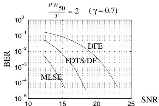
Figure 3: Simulation results of MLSE, FDTS/DF, and DFE
