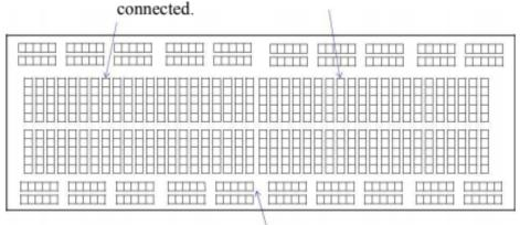
Every hole in this horizontal line is connected.
