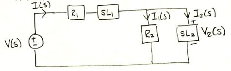
(b) (10 pts) What is H(s), the transfer function of this circuit relating the input v(t) to the output  $i_2(t)$ ? Express it as a ratio of polynomials in s.
