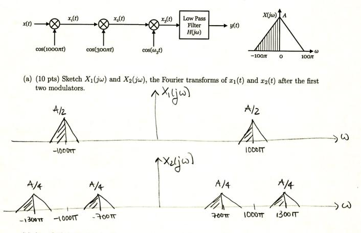
(b) (5 pts) If the goal is for the output y(t) to equal the input x(t), what is the lowest possible value of  $\omega_3$  to achieve this? (Note that  $\omega_3$  is the frequency of the third modulator.)
