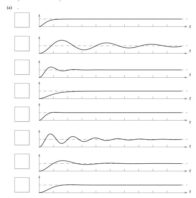
**PROBLEM 4.** Shown on the left are the step responses of eight second-order low-pass filters, labeled A through H. Shown on the right are the magnitude responses for these filters, but in a scrambled order. Match each magnitude response to its corresponding step response by writing a letter (A through H) in each answer box.
